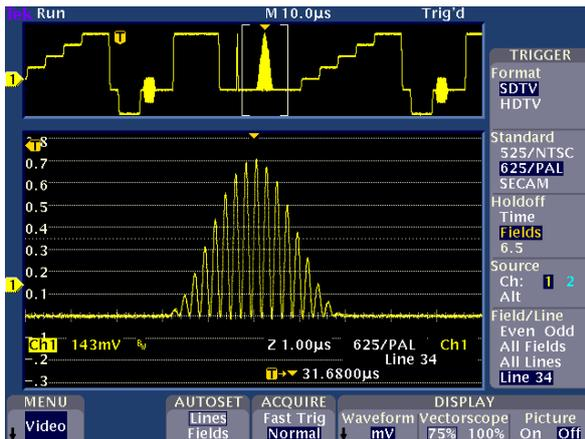
**OSD 870 fibre optic system Modulated 20T Pulse waveform with an almost perfect result.**
