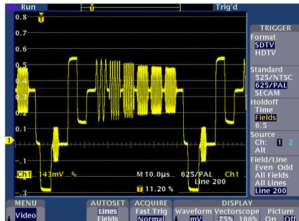
150 metres of RG59/U coaxial cable Multiburst waveform frequencies of 0.5 MHz, 1.0 MHz, 2.0 MHz, 4.0 MHz, 4.8 MHz and 5.8 MHz with the 4.8 MHz burst at -3.0 dB.
