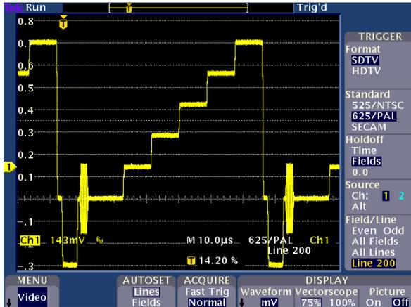
OSD 870 fibre optic system 5 Step Greyscale waveform which is very similar to the output of the test signal generator.
