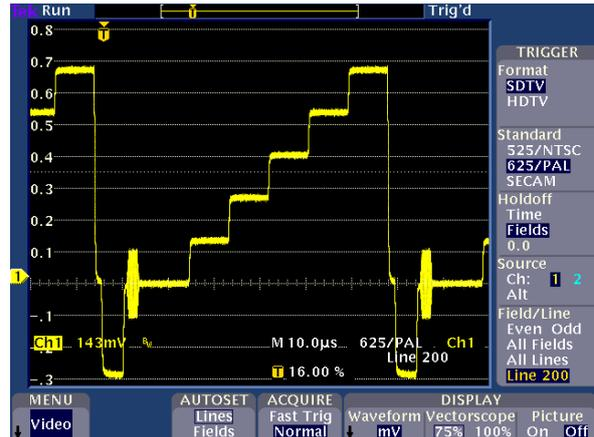
150 metres of RG59/U coaxial cable 5 Step Greyscale waveform showing low video level, rounding of the greyscale steps and horizontal sync pulse and low colour burst.
