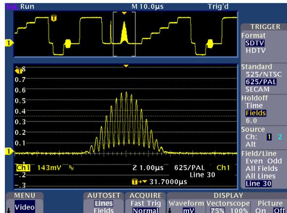
**150 metres of RG59/U coaxial cable Modulated 20T Pulse waveform showing video level loss and low chrominance to luminance amplitude.**
